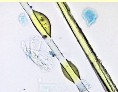
Yellow “batt” insulation
